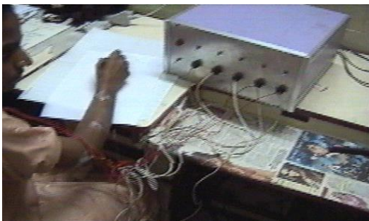
Fig 4: A close up of signal recording with indigenously developed EMG prototype
