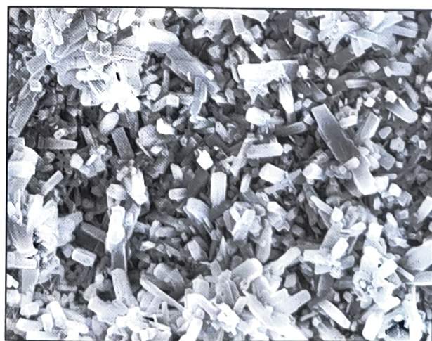
Micrograph 2A. Surface deposition of D/Sense2 varnish treated discs \times 2500 .
